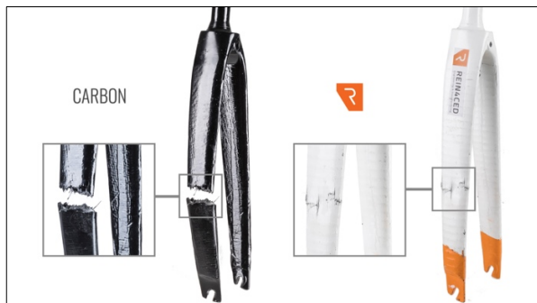
The disruptive impact-resistant material of REIN4CED eliminates the sudden and dramatic failure of carbon bicycle frames that put riders' lives in danger.
